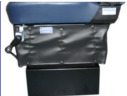
SideRiser fitted with protective Gaiter
